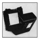
B. The film back frame, on the other hand, consists of a base with a dark slide slit and a back cover with a film type indicator frame. The film back frame completely encloses the film holder and shields it from outside light, as well as connecting it to the camera main body.
