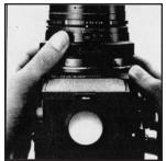
A. The lens is focused on the subject, by rotating the focusing ring in either direction, while checking the effect on the micro-prism / splitimage rangefinder spot in the center of the focusing screen (standard type).
