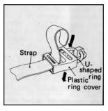
B. Next, insert the U-shaped ring into the slot of plastic cover.
