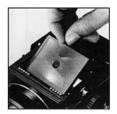
B. To install the focusing screen, insert the protrusions at the forward end of the focusing screen frame into the corresponding openings in the focusing screen frame of the main body. Then, drop the rear end of the focusing screen and slide the screen removal lever to the right.
