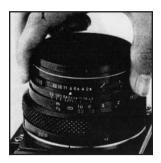
A. The aperture ring is rotated, in either direction, to set the required f/number opposite the white index dot. The aperture ring click-stops at the numbered settings. Intermediate settings are also possible.
