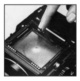
A. The focusing screen can be exchanged, depending on the type of photographic work being undertaken. First, remove the finder attached to the camera main body. Then, move the screen removal lever in the arrow-indicated direction, as illustrated. Finally, lift it up by the lever.
