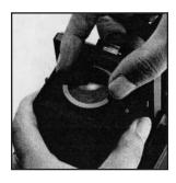
D. The standard magnifier supplied with the waist-level finder has a power of -1.5 diopters, which can be exchanged for others with powers of -4.5, -3.5, -2.5, -0.5, and +1.5 diopters. These optional accessories should be purchased to suit the user's eyesight, if necessary. Simply rotate the magnifier frame in the counter-clockwise direction to unscrew. Attach in the reverse manner.
