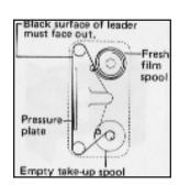
\* The spool holders on the left side will be locked securely, when the back cover is closed.
