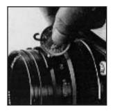
A. Unscrew the set screw on the time exposure lever until further revolution is not possible, which will permit the lever to be moved freely.
