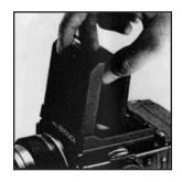
C. To close the focusing hood, first, push down the magnifier (if it is flipped up). Next, press in both side frames, as illustrated, and, at the same time, press the front frame back towards the rear end. The focusing hood will automatically be folded down.
