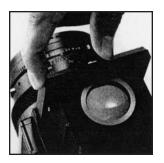
B. The magnifier can be flipped up into viewing position, by simply sliding the focusing hood/magnifier catch in the arrow-indicated direction (to the left). To return the magnifier to its storage position, simply push it down until it catches.
