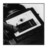
A. Depress the battery chamber button with your finger and at the same time, move the battery chamber cover in the arrow-indicated direction. The cover will come off easily.
