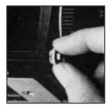
B. Safety Lock- The shutter release button has three settings to which it can be set by rotating in the clockwise direction. Two of these settings have safety-locking features of slight difference. The three positions are indicated by the red dot being placed at the bottom, at a position of 45° from bottom setting and at the side, with functions differing as per table.
