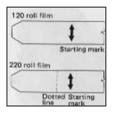
When loading 220 roll film in it's exclusive film back, do not mistake the dotted line for the starting point, as it is located before the arrow marks.
