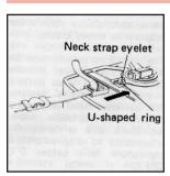
A. First, insert the U-shaped ring into the neck strap eyelet, as illustrated.
