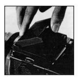
A. The focusing hood of the waist-level finder is opened by pushing or pulling up on the focusing hood/magnifier catch at the rear end of the folded waist-level finder.
